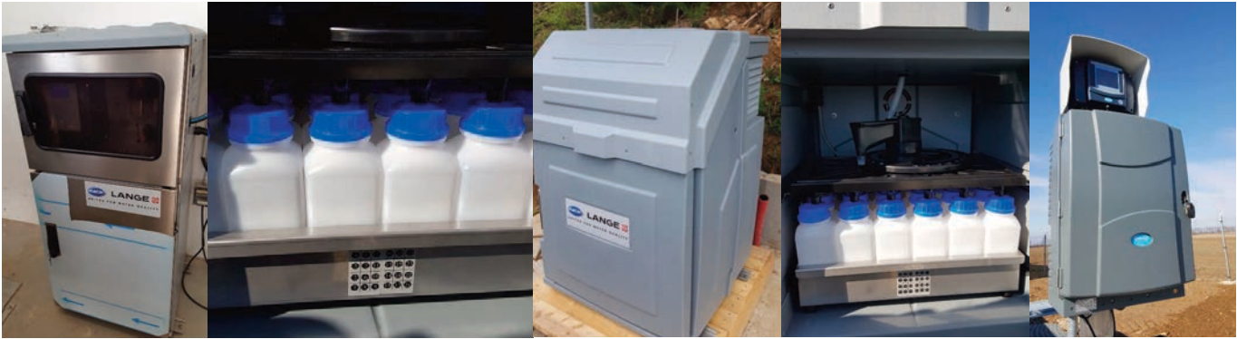
Fig. 2. Sampler for the daily and hourly collecting of the influent and effluent
